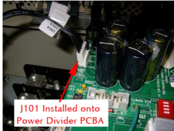
Figure 10 – Install power cable #0830763 into J101 of the Power/Divider PCBA, and the opposite end into J11 of the monitor box (note that J11 is not labeled on the monitor box, it is the left-most connector).
